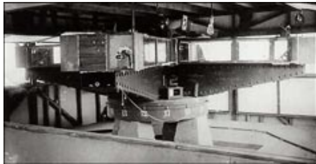
Figure 3: Miller's interferometer with an effective arm length of L = 32\text{m} achieved by multiple reflections. Used by Miller on Mt.Wilson to perform the 1925-1926 observations of absolute motion. The steel arms weighed 1200 kilograms and floated in a tank of 275 kilograms of Mercury. From Case Western Reserve University Archives.
